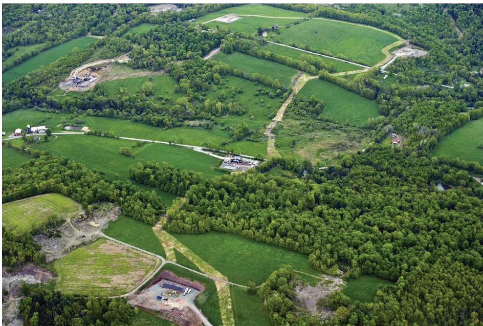
Aerial view of well pads, feeder pipelines, and access roads in Dimock, PA
